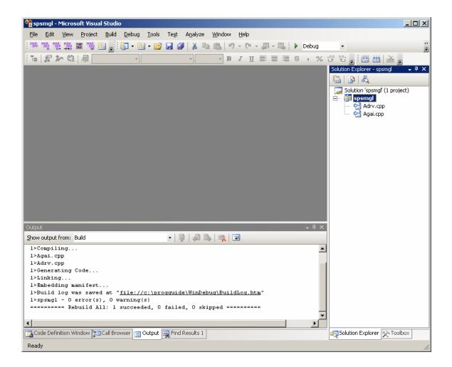
If the files are added correctly, they should appear under the solution spsmgl as per above. At this point users should build the model to ensure everything is working. This can be done using the drop down menu Build: Build spsmgl.
