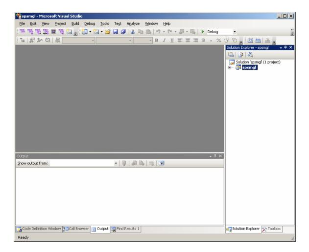
Before adding the selected files, make sure that the solution spsmgl is highlighted (see the right hand panel in the above snapshot), and that the solution tab is selected on the bottom of the solution panel.
